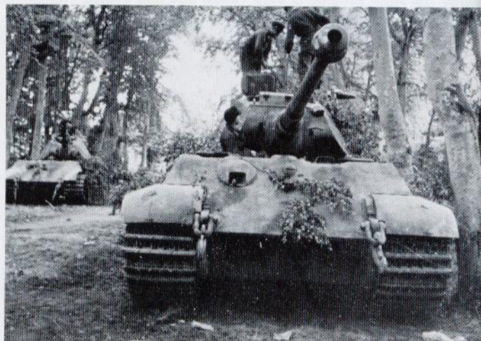
The 3rd company of sPzAbt 503 retained their Tiger I tanks during the campaign in Normandy. This is a late production version with the cast cupola and steel rimmed road wheels. The color scheme is a textbook application of Red Brown and olive green over a base of Dark Yellow. Note the battered condition of the few sheet metal mudguards that remain. (Bundesarchiv)
