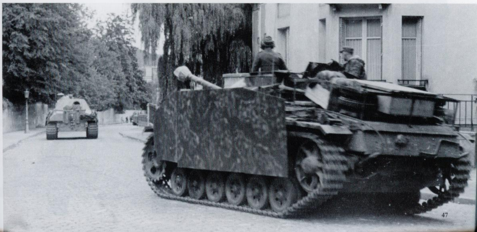
This StuG III shows a very heavy application of Olive Green and Red Brown over the Dark Yellow. Hardly anything remains of the base color. In common with many StuG III units, this "HG" vehicle carries considerable stowage on the engine deck, where it was out of the way. (Bundesarchiv)
