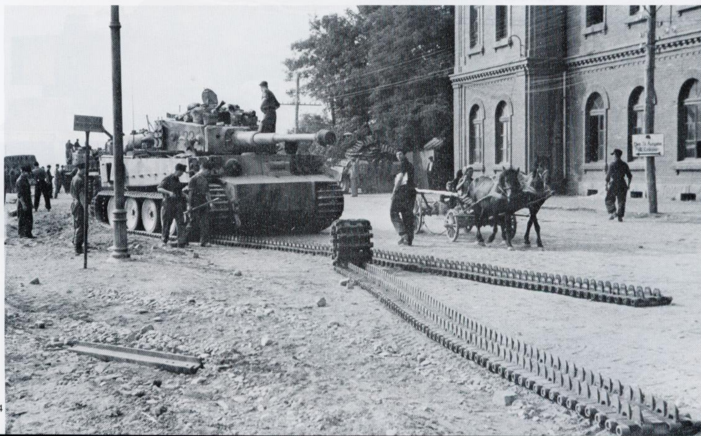
This early production Tiger I is seen in late 1943, still fitted with the Feifel air cleaners. The color scheme is Dark Yellow with some light mottling in Red Brown. The markings, in Black, denote the 2nd vehicle in the 1st company. The Tigers in each company carried the company letter ("A", "B", "C" for 1st, 2nd, or 3rd company), followed by the platoon and vehicle number of the standard three digit system. From early 1943 through the epic battle at Kursk, the Tigers of "GD" used an "S" prefix with the platoon and vehicle numbers following. (Bundesarchiv)
