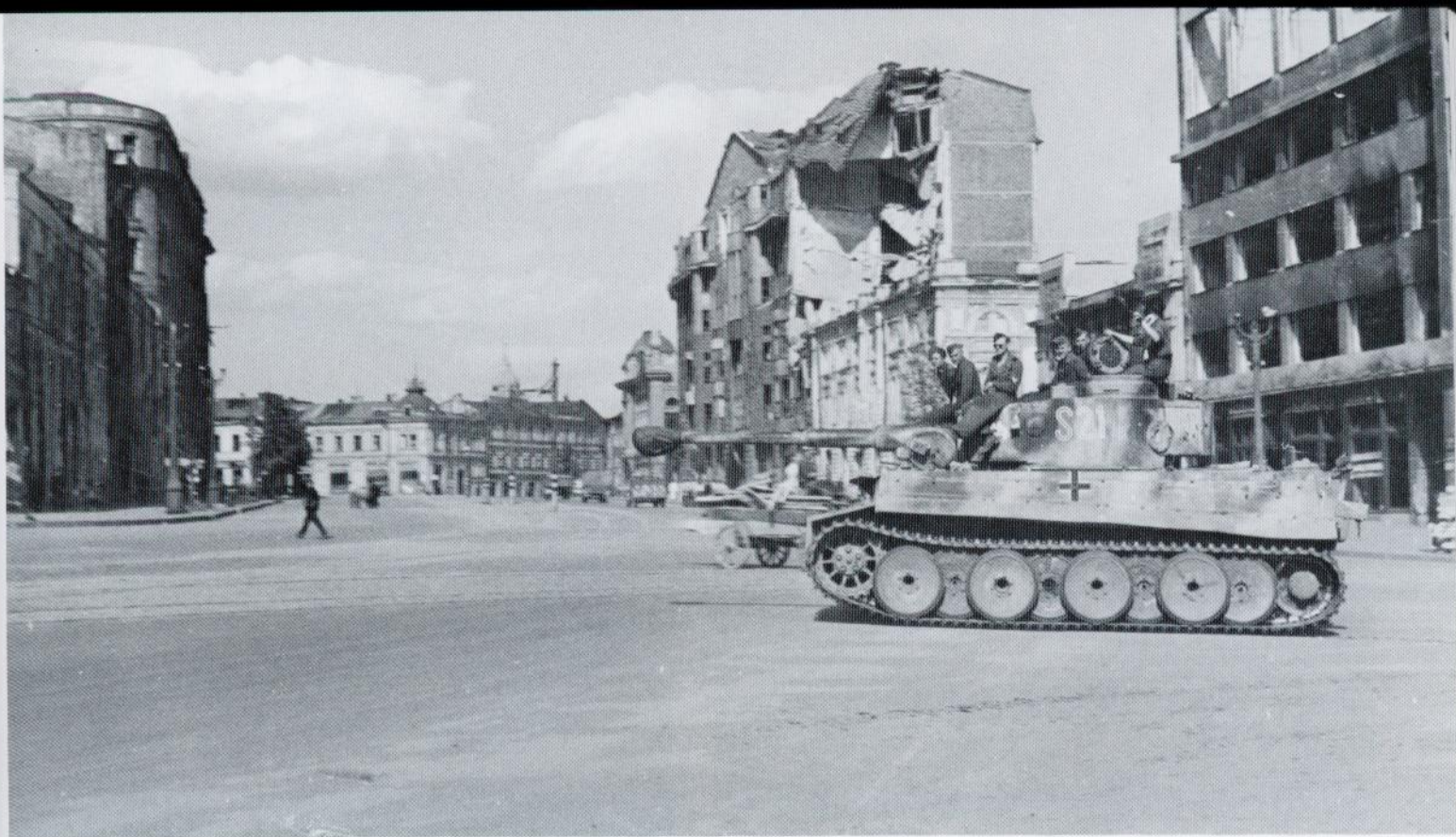
During the Kursk battle, German units fought in several towns and cities. This Tiger I of "Das Reich" is Dark Yellow with Red Brown and Olive Green mottling. The vehicle number is White. On the front turret side is the White gnome of the Tiger company. The Feifel air cleaners have been removed from this vehicle. (Bundesarchiv)
