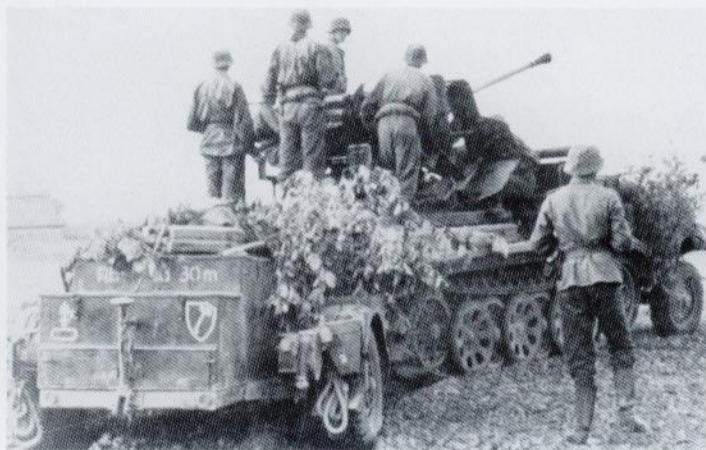
(Below) This SdKfz 6 self-propelled 3.7cm Flak 37 halftrack is seen in Russia during BARBAROSSA. The markings, in White, denote the 2nd self-propelled Flak battery. The division sign is the standard design used by "LAH" during the invasion of Russia. Note the distance warning in White. (NARS)
