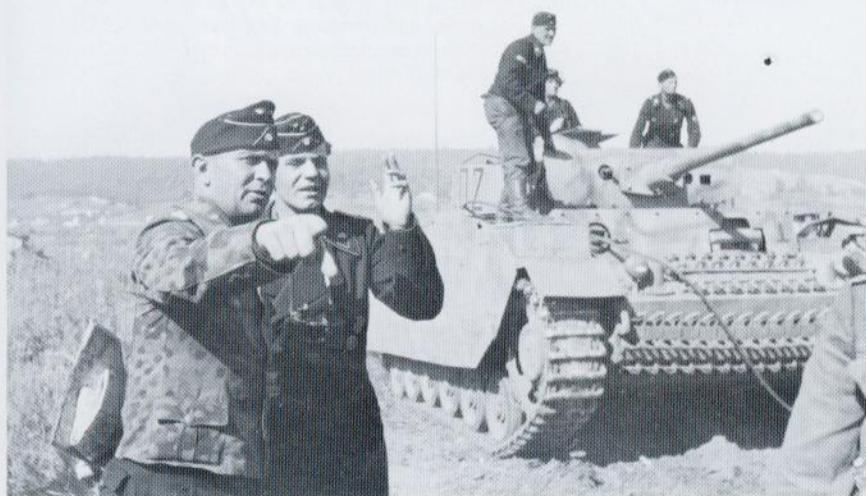
This late production PzKpfw III ausf M of 7th Panzer Division (Heer) carries the same temporary unit sign as 1st SS Panzer Grenadier Division Leibstandarte "Adolf Hitler". The sign is Black, and the turret numbers are Red with White borders. The base color is Dark Yellow with Red Brown overspray. (Bundesarchiv)
