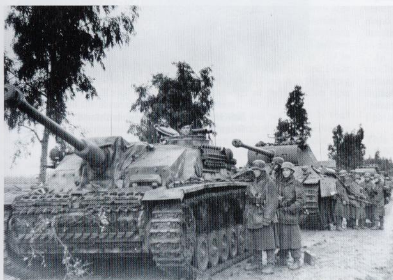
(Left) In 1944, "HG" adopted a very heavily applied three color scheme very similar to that seen on the previous page. This StuG III ausf G is Dark Yellow with Olive Green and Red Brown mottling. The tactical sign for a StuG unit is in White on the front mudguard. (Bundesarchiv)
