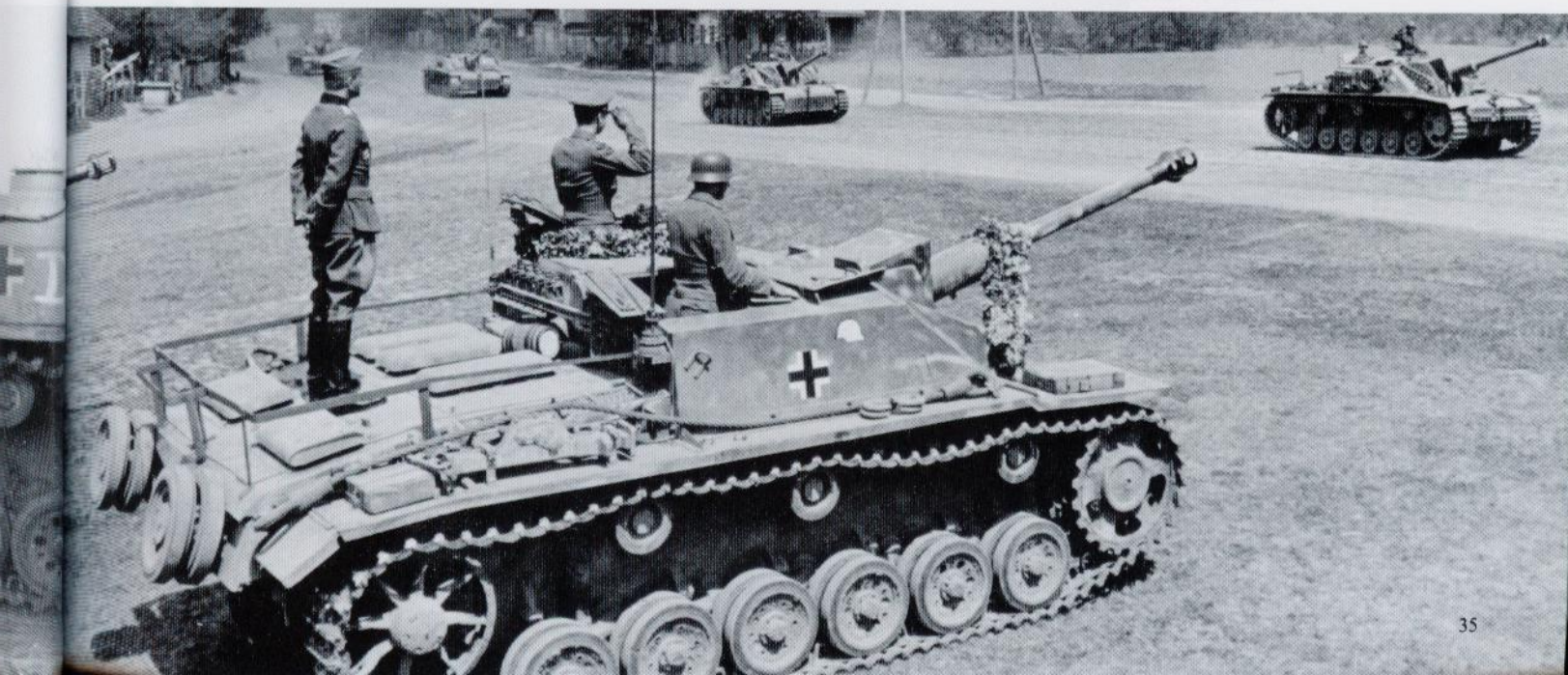
(Below) This is the StuG III ausf G of the commander of the "GD" StuG Abt. The color scheme is a very heavy mottling of Olive Green over a Dark Yellow base. Very little of the base color can still be seen. In common with most "GD" command vehicles, the helmet on this StuG III has a narrow Black outline over the top edge. (U. Feist)
