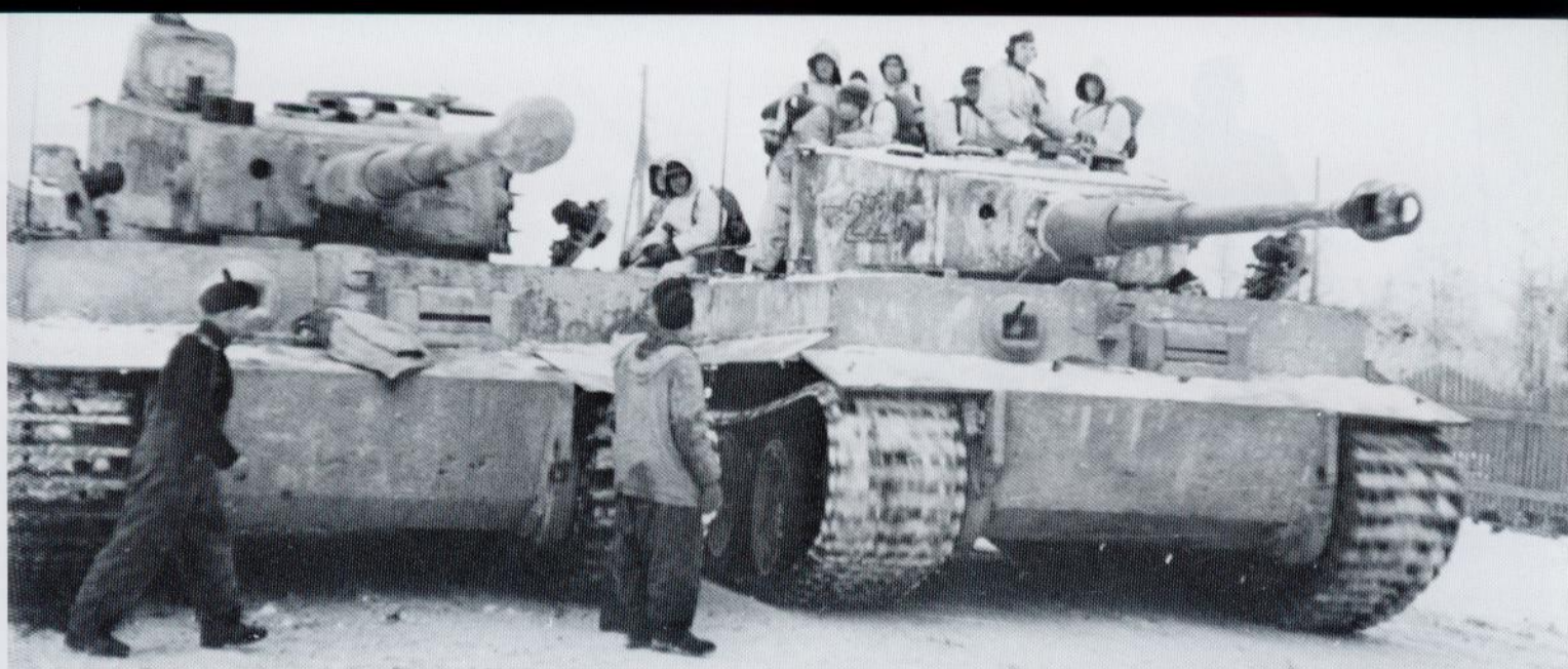
The winter of 1943-44 brought snow camouflage and newer Tiger Is. These Tigers have the later cast cupola and single headlight. The White temporary paint is somewhat rough, the usual case. The turret numbers are Yellow Ochre outlined in Black. (Bundesarchiv)
