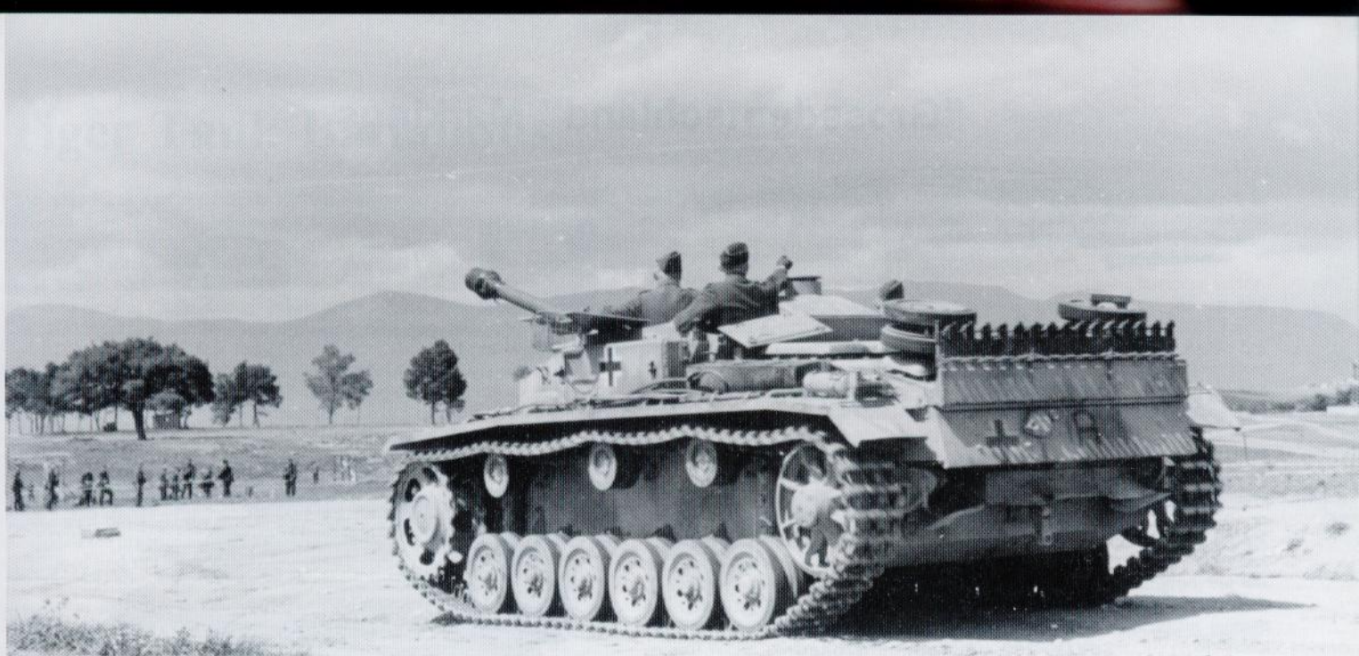
Another StuG III ausf F of "HG", seen in 1943, is overall Dark Yellow with a Black section letter "A". Note the wire cage mounted over the gunner's hatch sight opening, and the framework for the spare tracks on the rear deck. (Bundesarchiv)
