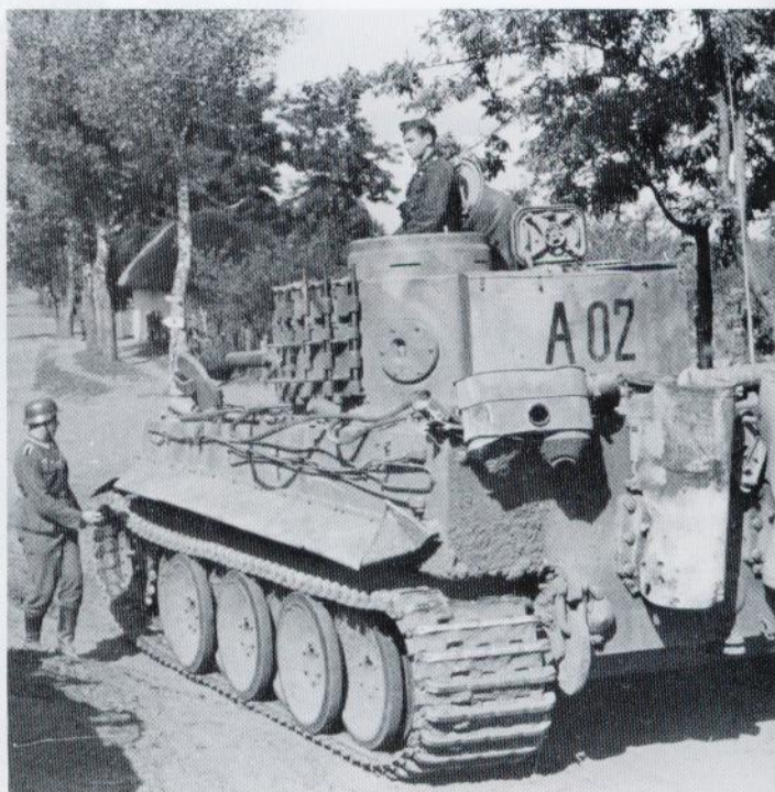
This early production Tiger I is seen in late 1943, still fitted with the Feifel air cleaners. The color scheme is Dark Yellow with some light mottling in Red Brown. The markings, in Black, denote the 2nd vehicle in the 1st company. The Tigers in each company carried the company letter ("A", "B", "C" for 1st, 2nd, or 3rd company), followed by the platoon and vehicle number of the standard three digit system. From early 1943 through the epic battle at Kursk, the Tigers of "GD" used an "S" prefix with the platoon and vehicle numbers following. (Bundesarchiv)
