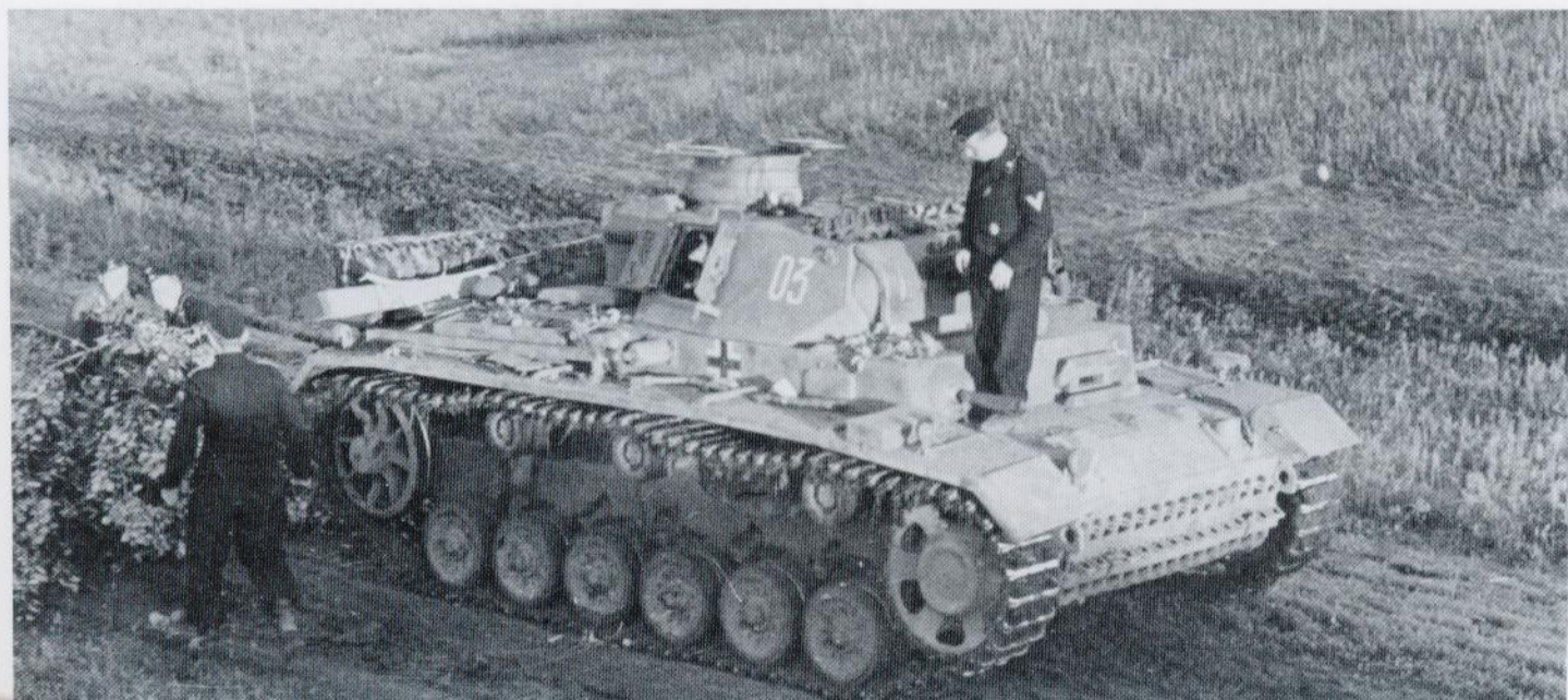
A PzKpfw III aust J of 16th Panzergrenadier Division carries the division sun wheel sign on a sprayed patch of darker color on a basic color scheme of Dark Yellow. The sun wheel and the tank turret number are both in White. A light random mottle of Olive Green has been applied to this vehicle. (Bundesarchiv)
