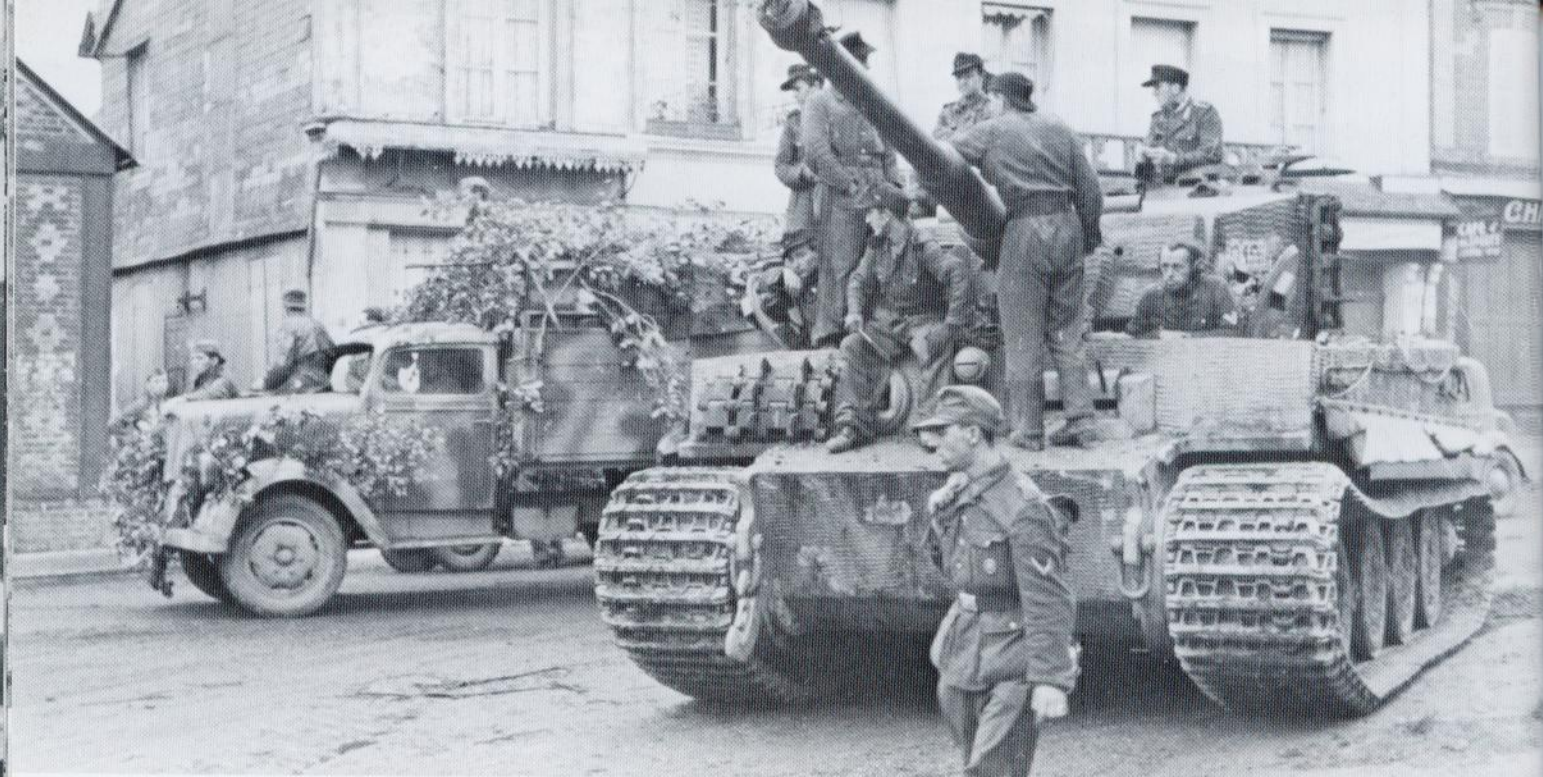
The 3rd company of sPzAbt 503 retained their Tiger I tanks during the campaign in Normandy. This is a late production version with the cast cupola and steel rimmed road wheels. The color scheme is a textbook application of Red Brown and olive green over a base of Dark Yellow. Note the battered condition of the few sheet metal mudguards that remain. (Bundesarchiv)
