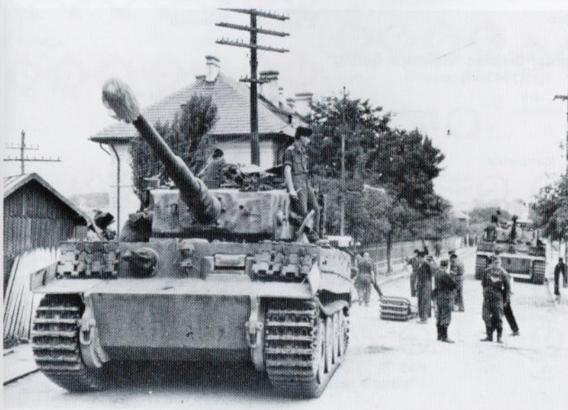
Another Tiger of "GD", seen during a track change, carries a Dark Yellow color scheme with a Red Brown overspray. As was common, this crew has gathered a number of extra items of equipment. The turret number, "A32", is Black.
