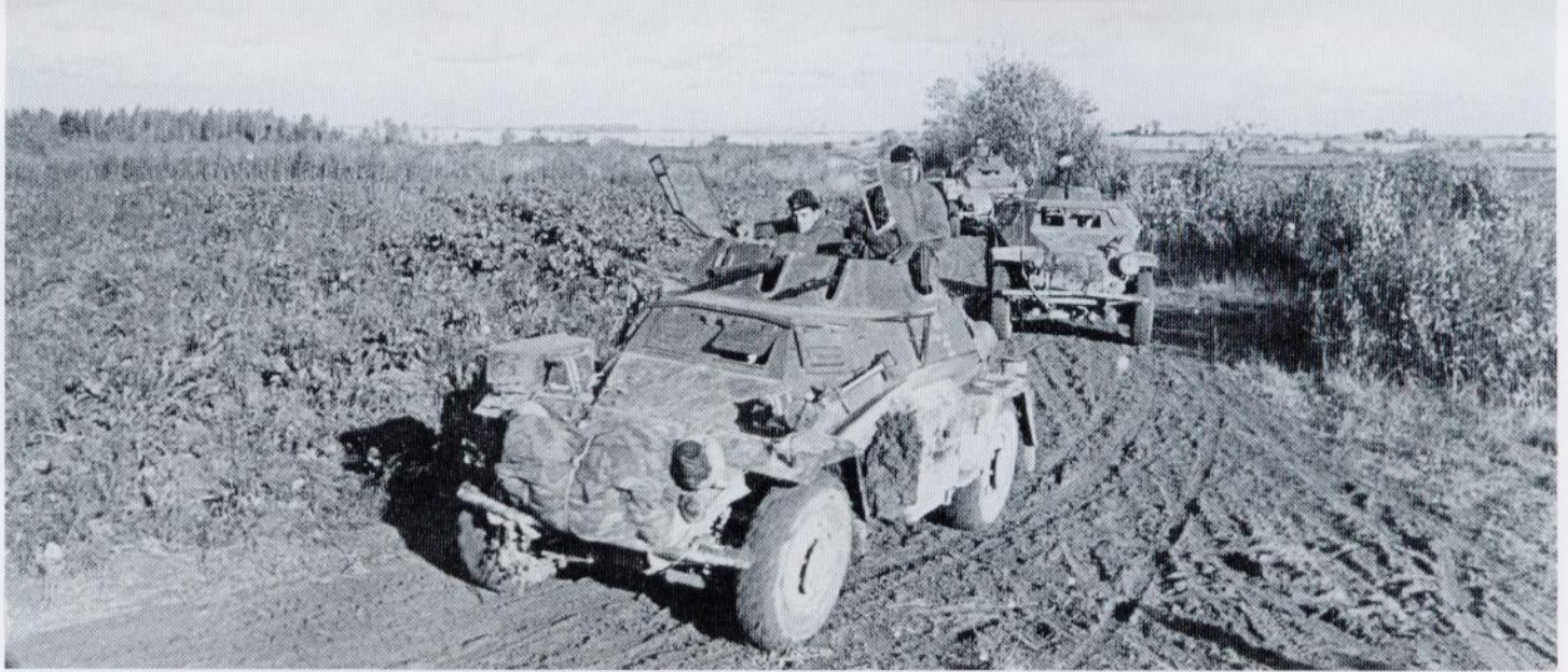
This column of SdKfz 222 armored cars of 36th Panzer grenadier Division shows the weathering effects of operating in the Russian campaign during rainy weather. The division symbol is painted in White on the side of the car, a good contrast against the Dark Gray paint. (Bundesarchiv)
