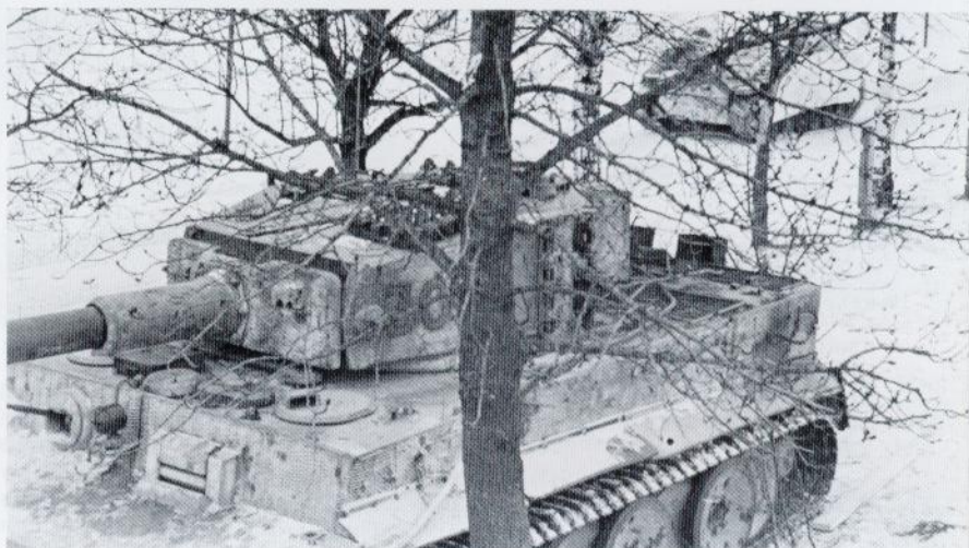
The winter of 1943-44 brought snow camouflage and newer Tiger Is. These Tigers have the later cast cupola and single headlight. The White temporary paint is somewhat rough, the usual case. The turret numbers are Yellow Ochre outlined in Black. (Bundesarchiv)
