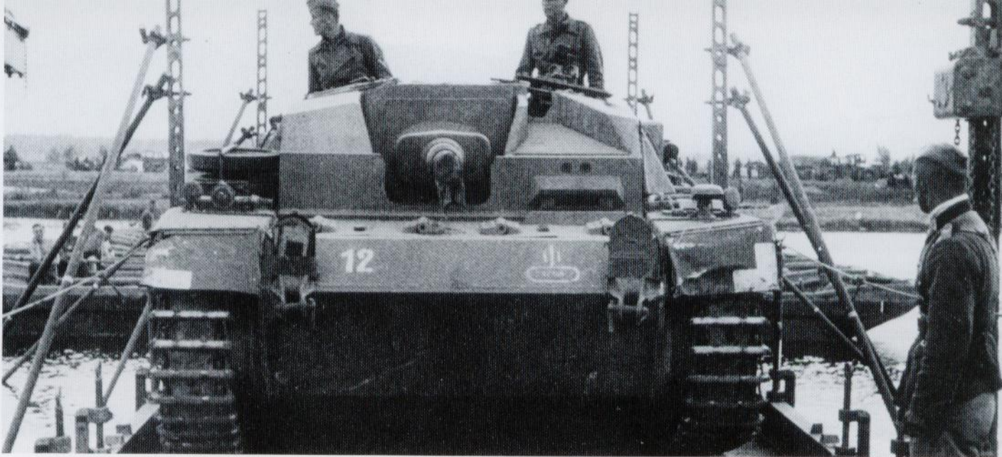
(Above) A StuG III of 203rd StuG Abt (Assault Gun Battalion) carries the tactical sign for a self-propelled gun unit in White. Inside the tactical sign is the designation of the battery, "3/203". The vehicle number and width markings are also White. (Bundesarchiv)
