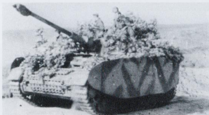
This PzKpfw IV ausf H does not carry a division sign, but is typical of vehicles in 1944. The Dark Yellow base color has been oversprayed with Olive Green. By 1944, superior Allied air power led to regular use of heavy foliage for better camouflage. (Bundesarchiv)
