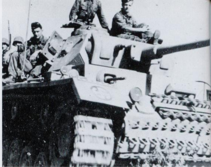
A PzKpfw III ausf J, seen in 1943, is overall Dark Yellow. The "Wiking" symbol is White on a Black disk. The turret numbers, covered with a heavy layer of dust, are Red with White outlines. (Bundesarchiv)
