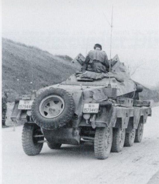
A late production SdKfz 232 armored car of 15th Panzergrenadier Division travels down a road in Sicily in support of "Hermann Göring" troops. The star mast radio antenna replaced the earlier conspicuous frame antenna. This vehicle has a light mottle of Red Brown and Olive Green. (Bundesarchiv)
