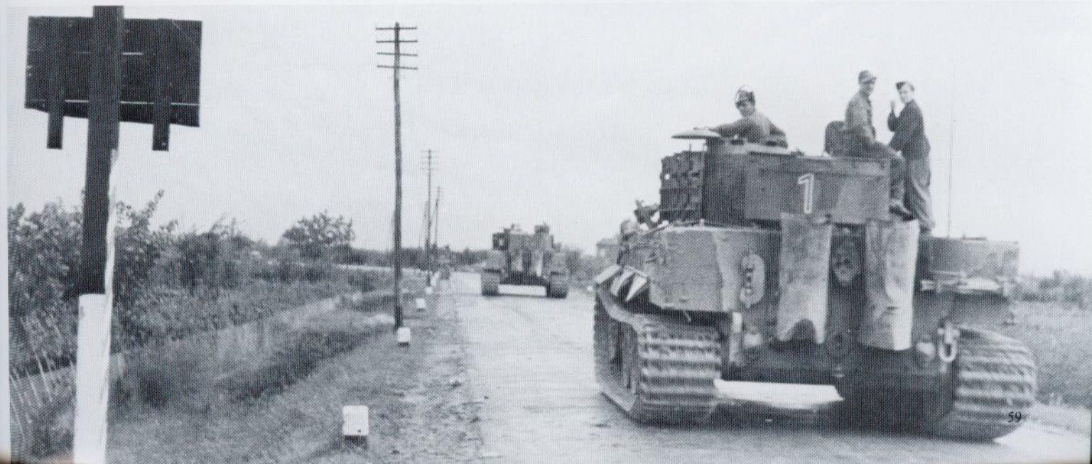
This Tiger I of sPzAbt 503 of PzRgt "Bake" shows the typical appearance of these late production models. The spare track shoes serve to increase the already effective armor. The color scheme is the Dark Yellow and Red Brown often used by this unit. Note the contrast between the wet and dry mud areas. (Bundesarchiv)
